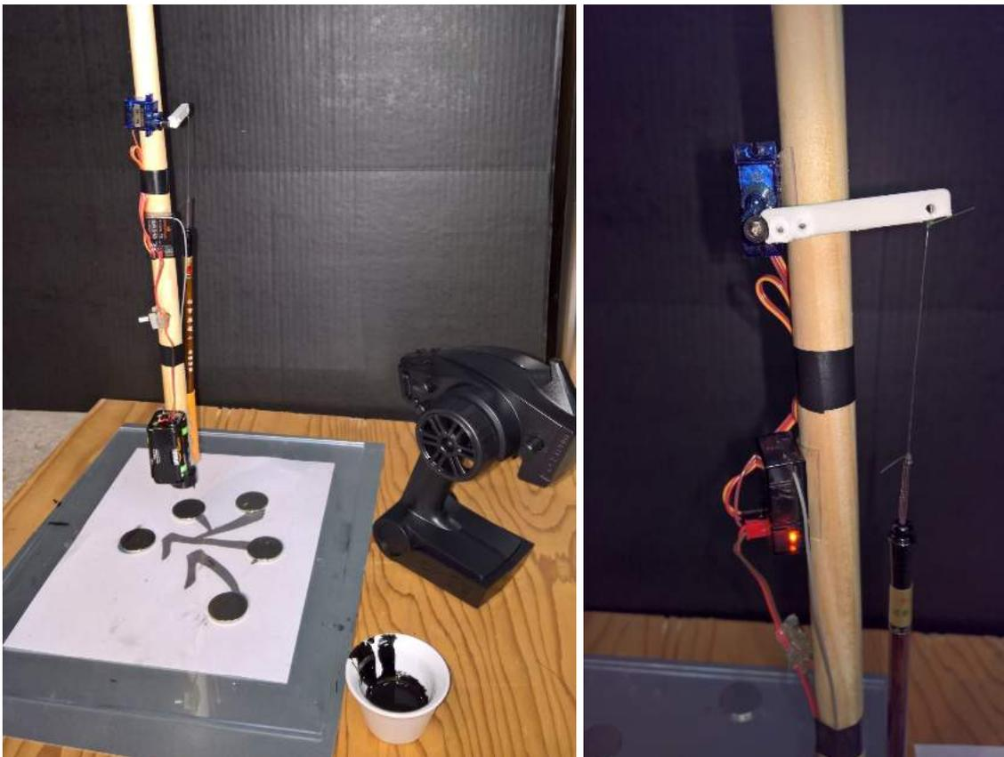
The pendulum uses a 1.2m solid wood rod. I've experimented initially with a suspension made from a bunch of hooks, but settled on a more flexible suspension made from fishing gear so it can rotate when needed. It is one of these physical facts that are omitted from the computer simulation. The magnets have a physical extend, and this causes the pendulum bar to "roll" around its axis in certain configurations.
